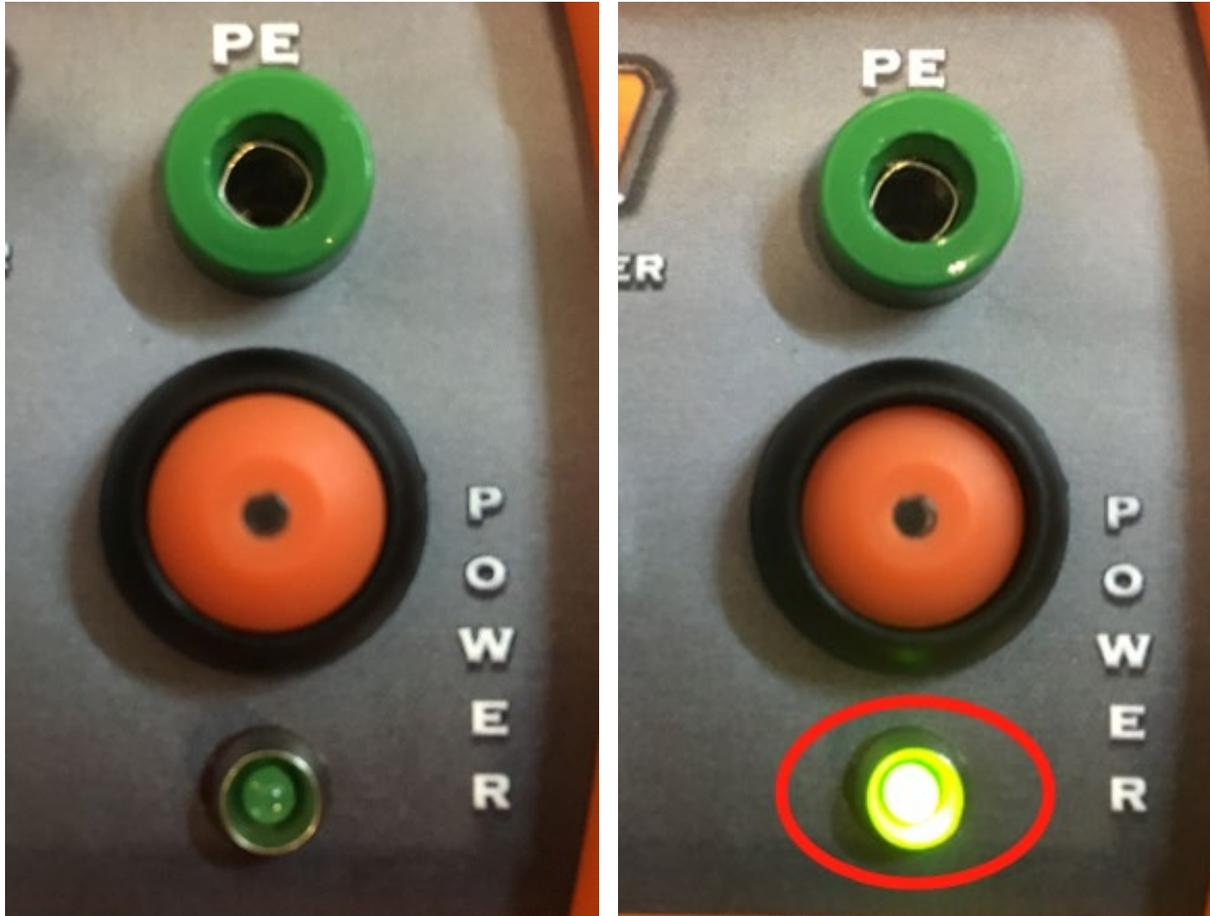
Once powered up, the **POWER LED** will light for 5 seconds, then flash every 5 seconds to indicate that the device is running properly.
